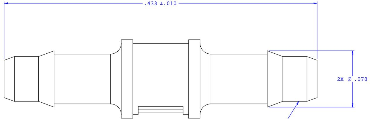
2X INSTRUMENT QUALITY PART. NO PARTING LINE PERMITTED ON THIS CONICAL SURFACE
